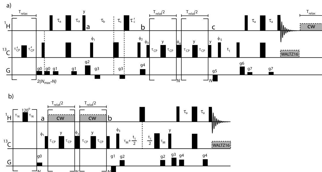
Figure 1. Pulse scheme for the measurement of methyl ^1\text{H} - ^{13}\text{C} (a) spin-state selective and (b) CW relaxation dispersion profiles. ^1\text{H} and ^{13}\text{C} pulses that are shown with the highest vertical bars are applied at the highest power levels possible. ^{13}\text{C} pulses during the constant-time CPMG element, including the flanking 90^\circ pulses are applied with a field strength of 16–17 kHz, with ^{13}\text{C} decoupling during acquisition achieved with a 2 kHz WALTZ-16 field. 39 The ^1\text{H} 180^\circ pulse that is applied during the multiplet selection element between points a and b of scheme (a) is of the composite variety 29 ( 90_x210_y90_x ). All pulses are applied along the x -axis unless indicated otherwise. The durations \tau_a and \tau_b are set to <1/(4J) (1.8 ms) and 1/(4J) (2.0 ms), respectively, where J is the one-bond ^1\text{H} - ^{13}\text{C} scalar coupling constant ( \sim 125 Hz), \tau_c = \tau_b - \Delta/2 and \tau'_c = \Delta/2 . N is any integer. Scheme (a): Delays \tau_{\text{eq}} = 2 –5 ms were inserted immediately after gradients g_4 and g_5 to ensure that the relative amounts of magnetization of each state faithfully reports on equilibrium populations. In order to separate each multiplet component into a separate subspectra the approach of Kontaxis and Bax is employed 29 where four separate spectra, A–D, are acquired with the (\phi_2, \Delta) set to (x, 0) , (y, 1/(6J)) , (-x, 1/(3J)) and (-y, 1/(2J)) , respectively. These spectra are subsequently manipulated post acquisition to produce the linear combinations A+2B+2C+D , A+B-C-D , A-B-C+D , and A-2B+2C-D which result in subspectra containing the isolated \beta\beta\beta , \alpha\beta\beta , \alpha\alpha\beta , and \alpha\alpha\alpha multiplets, respectively. The phase cycle is: \phi_1 = 2(x, -x), 2(-x, x) , \phi_3 = 2(x), 2(-x) , \phi_4 = x, -x , \phi_5 = 2(x), 2(-x) , \phi_{\text{rec}} = 2(x, -x), 2(-x, x) . Quadrature detection in F_1 is achieved via STATES-TPPI 40 of \phi_5 . Durations and strengths of the z -axis gradient pulses are (ms, G/cm), g_0 = (0.5, 4) , g_1 = (0.3, 5) , g_2 = (1.0, 25) , g_3 = (0.1, -4) , g_4 = (1.5, 6) , g_5 = (1, -17) , g_6 = (0.3, 12) , g_7 = (0.2, 8) . When \tau_c > \tau'_c the second gradient g_3 is applied as shown; otherwise, g_3 is applied during the \tau'_c duration. A ^1\text{H} CW field was applied for a duration T_{\text{relax}} immediately after acquisition to ensure the same degree of heating as in experiments recorded with scheme (b). Immediately prior to the first INEPT transfer 41 a ^{13}\text{C} CPMG element is applied, again to ensure uniform heating. N_{\text{max}} is the maximum value of N and \tau'_{\text{CP}} = T_{\text{relax}}/(4(N_{\text{max}} - N)) . The ^1\text{H} carrier frequency is placed in the center of the methyl spectrum and then jumped to 4.7 ppm after gradient g_6 . Scheme (b): Many details are as for scheme (a) and are not repeated. The ^1\text{H} 180^\circ pulse applied during the ^{13}\text{C} acquisition period is (90_x180_y90_x) . 29 Delays \tau_{\text{eq}} = 2 –5 ms were inserted immediately after g_1 and g_3 , \tau_m = 770 \mu\text{s} , \tau_N = 2.5 ms, N_C = 400 . ^1\text{H} CW decoupling during the CPMG interval was achieved as described in the text and previously. 42 The carrier is placed at 4.7 ppm for the duration of the ^1\text{H} saturation period (composed of 120^\circ pulses), 43 jumped to the methyl region of the spectrum and returned to 4.7 ppm after gradient g_3 . The phase cycle is: \phi_1 = x, -x , \phi_2 = 4(x), 4(-x) , \phi_3 = 2(x), 2(-x) , \phi_{\text{rec}} = x, 2(-x), x . Quadrature detection in F_1 is achieved via STATES-TPPI 40 of \phi_3 . Durations and strengths of the z -axis gradient pulses are (ms, G/cm), g_0 = (1, 5) , g_1 = (0.5, -15) , g_2 = (0.1, 10) , g_3 = (0.6, 12) , g_4 = (0.3, 12) . If N = 0 , a ^1\text{H} CW decoupling field of duration T_{\text{relax}} is applied after acquisition to maintain a constant level of sample heating.
